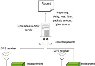
Figure: Structure of IP Measurement System
